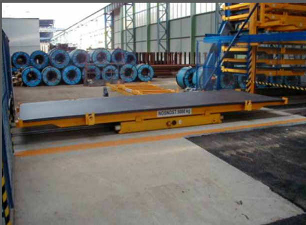
▲ Trolley with positioning device for rail unit bogie wheels.
