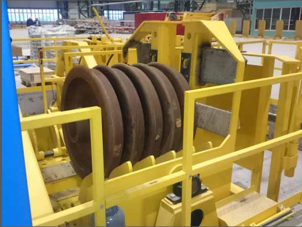
▲ Trolley with positioning device for rail unit bogie wheels.
